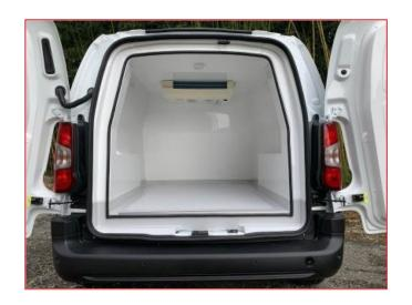
Power 0° is an invisible refrigeration unit in a temperature range of +0°C/+10°C in ATP conditions, designed for the transport of special goods for Small and Medium vehicles with a cargo room from 3 to 12 m<sup>3</sup>.
